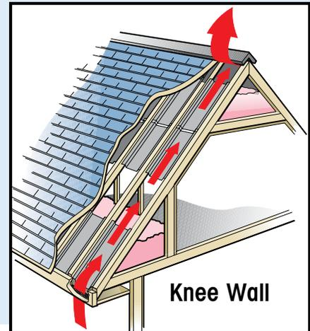
Maintaining an unrestricted air passageway between the soffit and ridge is crucial to the performance of the vent system, and must not be blocked or
