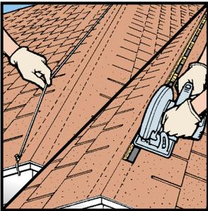
1. Measure a 3" slot, 1 1/2" each side of ridge centerline. This allows for a 2x ridge board or smaller. Snap chalk lines the entire length of the ridge. Cut slot with a circular saw and clean out debris. **Set saw depth so as not to cut roof rafters.** Stop the slot 12" short of any ridge end, intersecting ridge or obstruction (such as a chimney).
