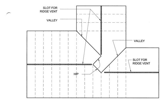
FIG 3. ROOF DIAPHRAGM PLAN VIEW - REALISTIC COMPLEXITY
