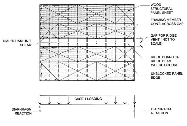
FIG 1. DIAPHRAGM PLAN VIEW - LOAD DIRECTION 1
