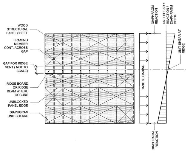
FIG 2. DIAPHRAGM PLAN VIEW - LOAD DIRECTION 2
