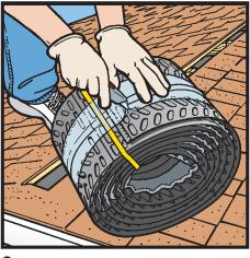
**2.** Cut clear band around roll, leaving colored band to hold all but the starter section together. Vent installs with legs down and flat cap on top.
