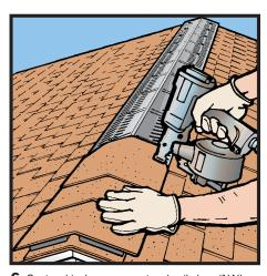
**6.** Center shingle cap on vent and nail along "NAIL HERE" guideline. Continue applying caps until all vent is covered with ridge caps. Do not overdrive nails. Nail head should be flush with top of shingle, without indenting it. Pre-forming caps in cold weather helps avoid cracking.
