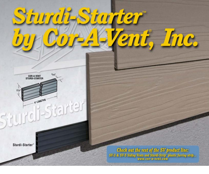
**Sturdi-Starter**<sup>TM</sup> is a 4-foot long x  $1^1/4^{T}$  wide x  $5/16^{T}$  thick (8 mm) profile extruded polypropylene plastic strip used as a starter strip behind the first course of fiber cement siding. Sturdi-Starter<sup>TM</sup> replaces strips ripped from good planks of siding, saving the installer money and materials, time on the job and extra labor.
