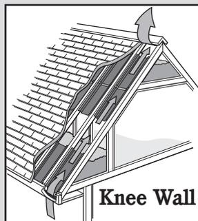
Maintaining an unrestricted air passageway between the soffit and ridge is crucial to the performance of the vent system, and must not be blocked or restricted. COR-A-VENT recommends a minimum 2" air space between the roof sheathing and vent chute or insulation
